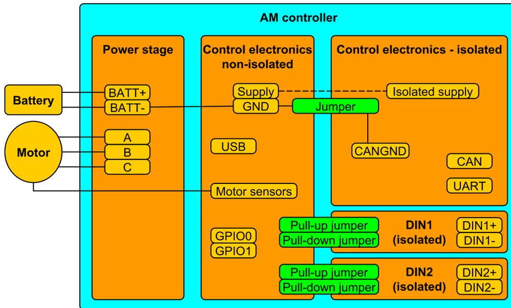
Figure 9.2: Block schematic of galvanic isolation
