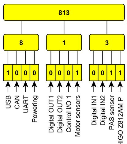
**Letter E – Other combinations of connectors** If the letter on position *Signal connectors type* is E, Other combination of connectors is used. Available combinations of connectors are listed in table 3.6. JWPF stands for usage of JST JWPF connector, 2.54 stands for usage of standard connector with pitch 2.54 mm (servo plug).
