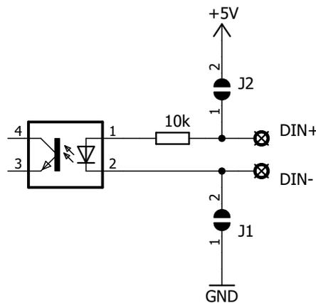
Figure 9.4: Digital input solder jumpers
