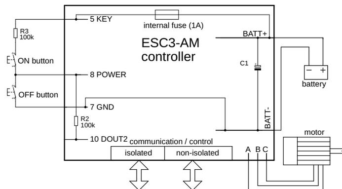
Figure 8.5: Two buttons powering scheme
