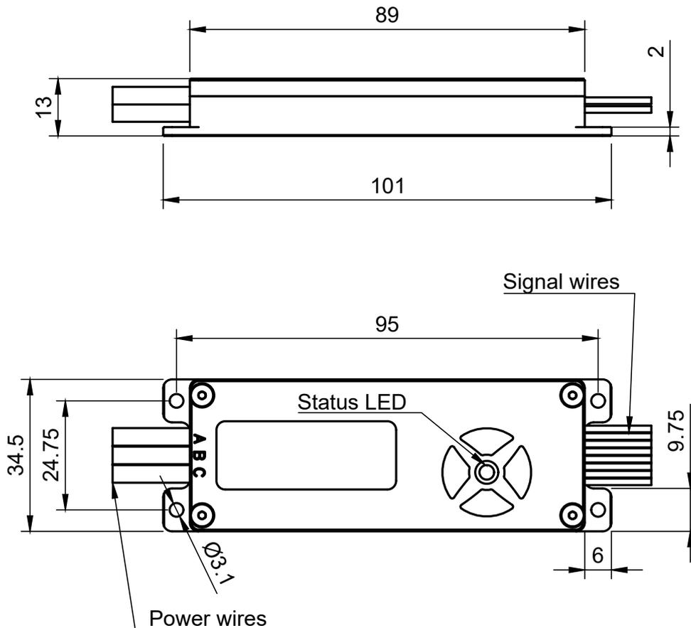
Figure 5.1: Aluminium housing for AM controller
