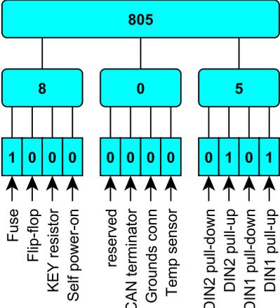
Note 1: When selected, CANGND and GND connected together – galvanic isolation is not present
