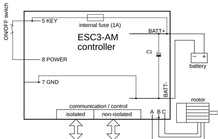
Figure 8.4: ON/OFF switch powering scheme
