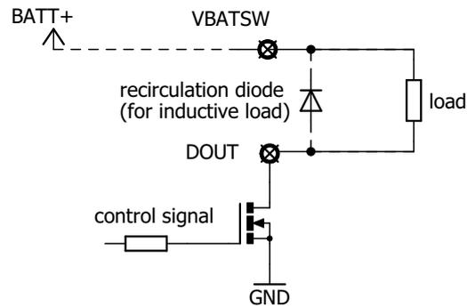
Figure 9.6: Digital output connection – open drain
