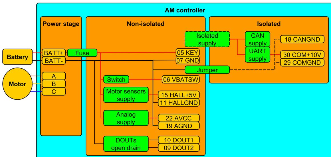
Figure 9.1: Block schematic of controller power supplies
