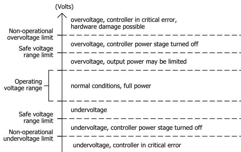
Figure 4.1: Controller voltage limits
