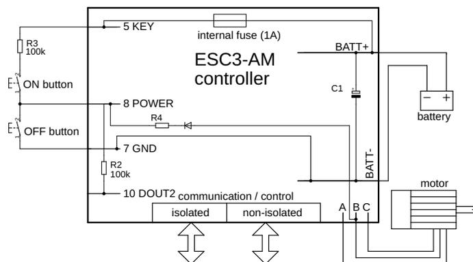
Figure 8.6: Two buttons powering scheme
