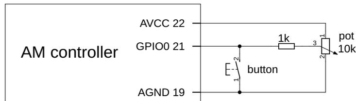
Figure 9.5: Connection of potentiometer and pushbutton to the same GPIO
