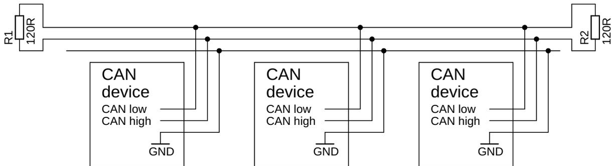
Figure 9.3: Connection of CAN Bus
