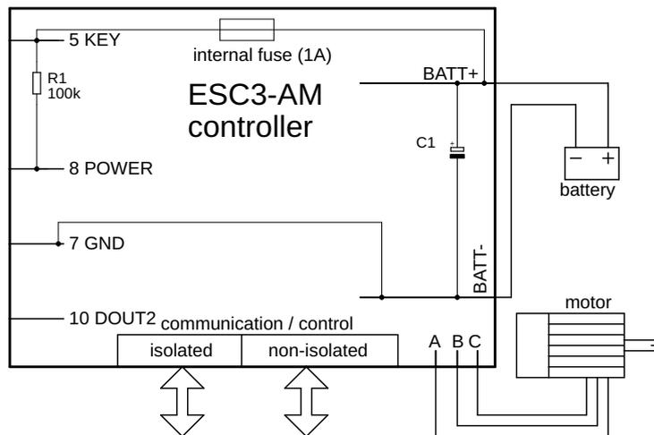
Figure 8.3: Constant on powering scheme
