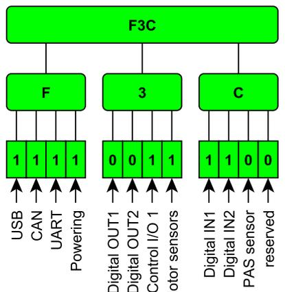
The diagram illustrates the binary encoding for the MPN F3C. The letter 'F' corresponds to a binary value of 1111, indicating the presence of USB, CAN, UART, and Powering connectors. The digit '3' corresponds to 0011, indicating the presence of Digital OUT1, Digital OUT2, Control I/O 1, and Motor sensors. The letter 'C' corresponds to 1100, indicating the presence of Digital IN1, Digital IN2, PAS sensor, and reserved connectors.
